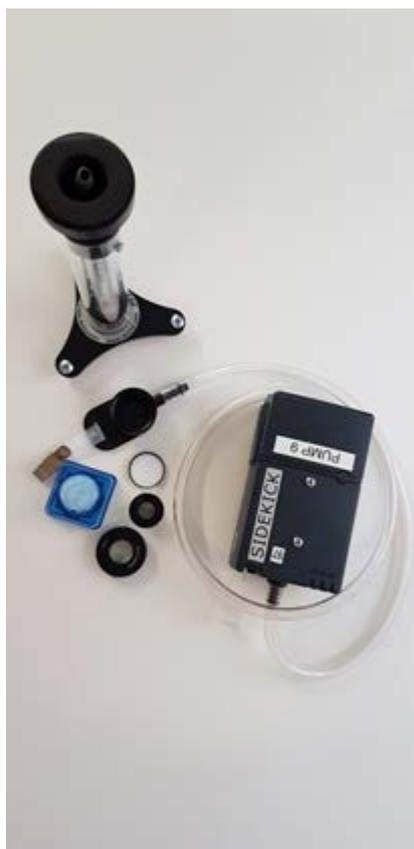
Figure 3. Sampling equipment used to test airborne LAA levels.
