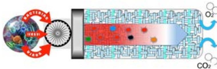
Figure 2. Contaminated air is drawn into the Biokker, this air then passes through a matrix of TiO<sub>2</sub> (Titanium Dioxide) and ZrO<sub>2</sub> (Zirconium dioxide) both naturally occurring materials that make up the catalyst in the system which is irradiated by Ultra Violet C lamps. The bound organic material is oxidised resulting in CO<sub>2</sub> / H<sub>2</sub>O as the only by-product.
