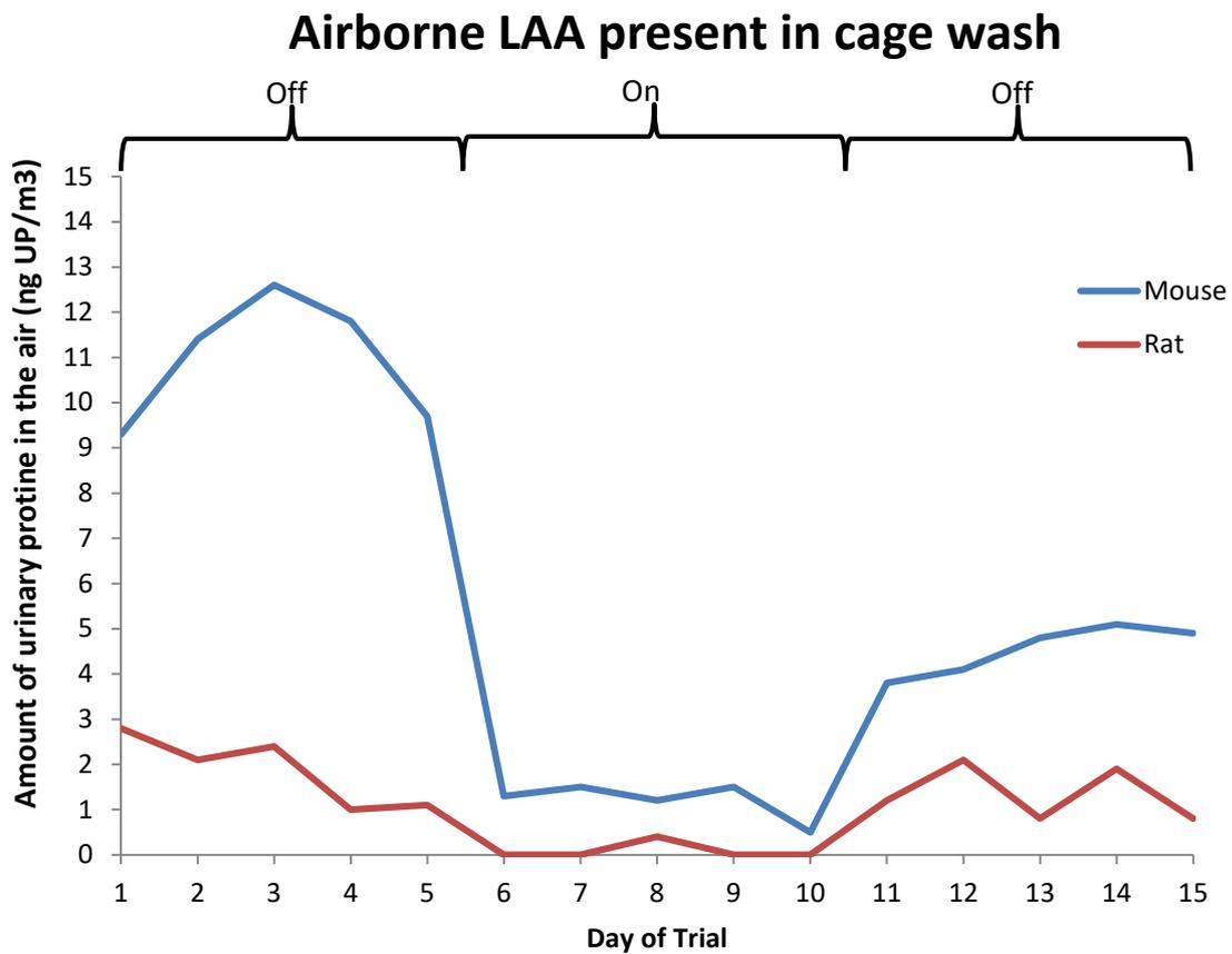
Figure 6. The amount of mouse and rat urinary proteins present in the air during trial days.
