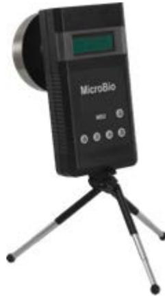
Figure 4. Parratt Microbio MB2 sampler used to measure air microbiology.
